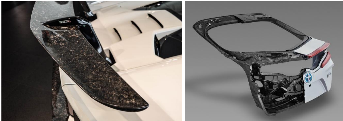
Figure 1. Rear wing of the Lamborghini Huracan Performante (left) [19]; Rear door frame of the Toyota Prius PVH [15]
